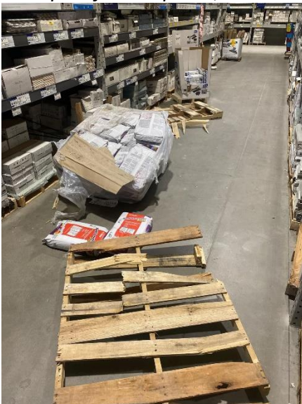
Example of a bad pallet, that should not be shipped (e.g., broken slats, decaying wood)
